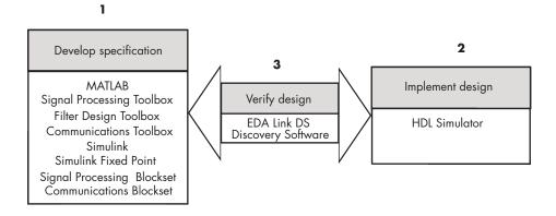
As the figure shows, EDA Simulator Link DS software connects tools that traditionally have been used discretely to perform specific steps in the design process. By connecting these tools, the link simplifies verification by allowing you to cosimulate the implementation and original specification directly. This cosimulation results in significant time savings and the elimination of errors inherent to manual comparison and inspection.
