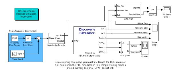
The HDL Cosimulation block models a Manchester receiver that is coded in HDL. Other blocks and subsystems in the model include the following:
