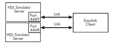
When you link the HDL simulator with a Simulink application, the simulator functions as the server. Using the EDA Simulator Link DS communications interface, an HDL Cosimulation block cosimulates a hardware component by applying input signals to and reading output signals from an HDL model under simulation in the HDL simulator.
