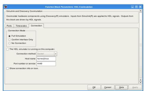
simulator running on the same computer, communicating in TCP/IP socket mode over TCP/IP port 4449.
